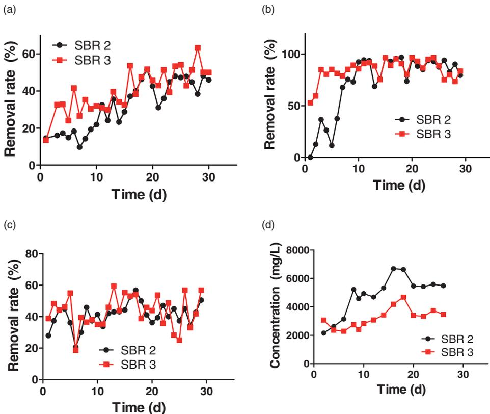
**Figure 6.** SBR operation performance for concentrate management. (a) COD removal efficiency (%), (b) ammonia removal efficiency (%), (c) SS removal efficiency (%), and (d) MLSS concentration. Note that both SBR 2 and SBR 3 were inoculated with acclimated activated sludge. SBR 2 was fed by a mixture of raw wastewater and concentrate while SBR 2 was fed by raw wastewater only.
