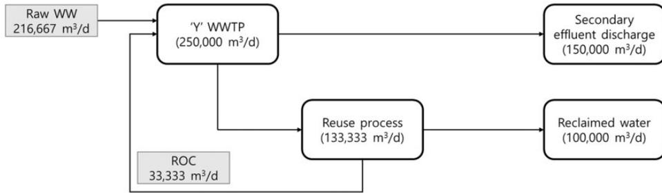
**Figure 2.** Mass balance of wastewater reuse process assuming 100,000 m<sup>3</sup>/d production of reclaimed water.
