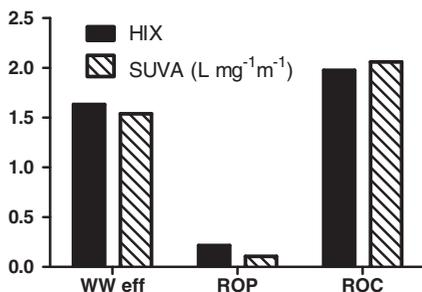
**Figure 4.** Humification index and  $SUVA_{254}$  for water samples. WW eff: secondary effluent; ROP: RO permeate; ROC: RO concentrate.
