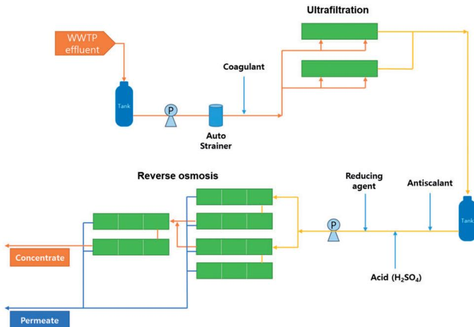
**Figure 1.** Schematic diagram of wastewater reuse process. The ROC is assumed to return as WWTP influent.
