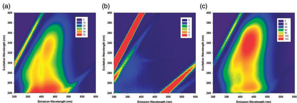
**Figure 3.** Excitation–emission diagrams for (a) secondary effluent, (b) RO permeate, and (c) RO concentrate.
