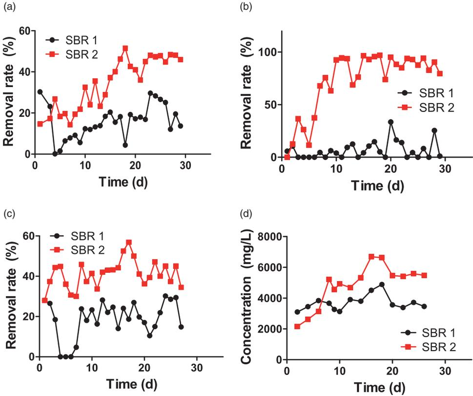
**Figure 5.** SBR operation performance for concentrate management. (a) COD removal efficiency (%), (b) ammonia removal efficiency (%), (c) SS removal efficiency (%), and (d) MLSS concentration. Note that a mixture of raw wastewater and concentrate was the influent for both SBR 1 and 2. SBR 1 was inoculated with unacclimated activated sludge while SBR 2 was inoculated with acclimated sludge.
