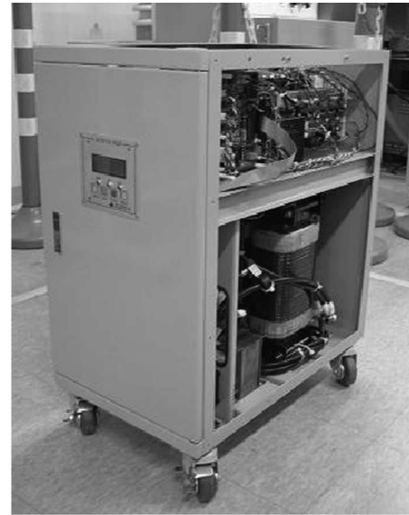
Fig. 12. Photograph of the proposed hybrid filter for 50-kVA load.
