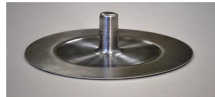
Fig. 12. Tube fabrication by spinning utilizing elastomer [194].
