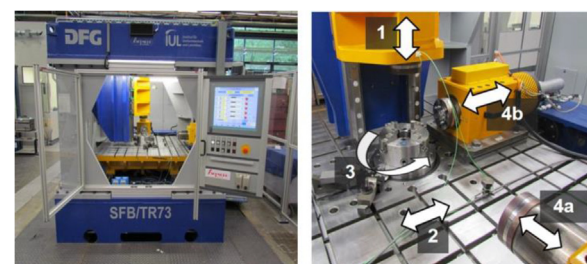
Fig. 28. Five-axis forming press for the incremental sheet-bulk metal forming [180].
