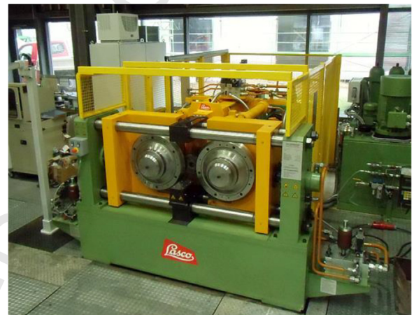
Fig. 31. Prototype machine for axial feed cross rolling [190].
