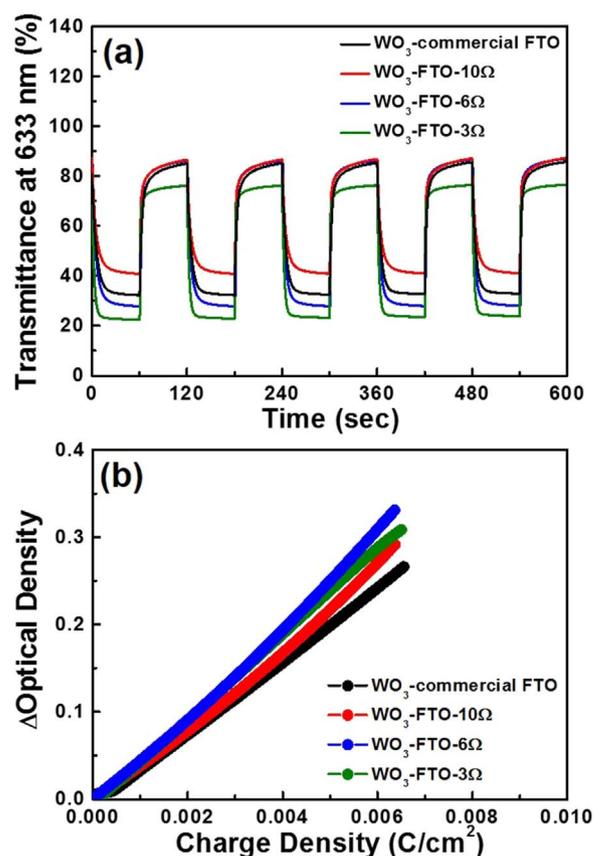
Fig. 7. (a) *In situ* optical transmittances spectra of the EC electrodes with all FTO films applied with an interval of 60 s at the potential of  $-0.7$  for colored state and  $1.0$  V for bleached state and (b) variation of OD at 633 nm with intercalated charge density at  $-0.7$  V.
