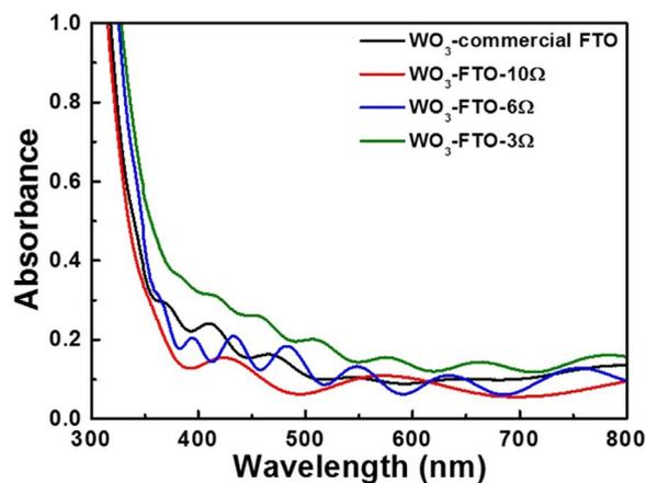
Fig. 5. Absorption spectra in wavelength range of 300–900 nm obtain from all WO<sub>3</sub>-FTO electrodes.
