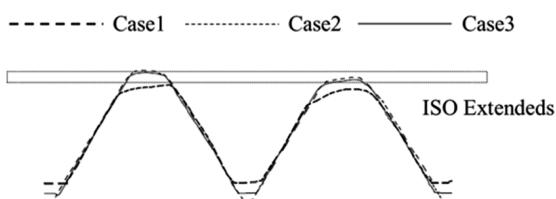
Fig. 11 Comparison of the thread profiles for three cases
