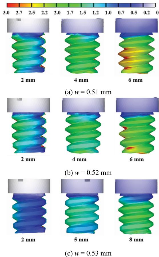
Fig. 7 Stepwise deformed shapes and effective strain distributions according to the die gap (Case 2)
