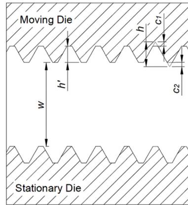
Fig. 2 Design parameters related to thread rolling dies
