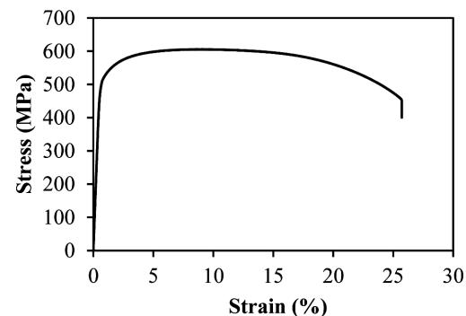
Fig. 3 Stress-Strain curve for the Titanium Grade2 wire
