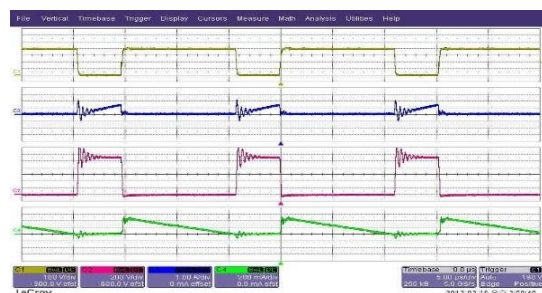
Figure 5. Switching voltage-current, diode voltage-current
