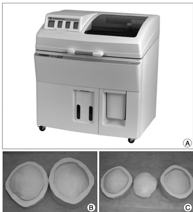
Figure 8. PMMA fabrication for cranioplasty using 3D printing, with (A) the 3D printer, (B) the prefabricated mold, and (C) the resultant PMMA cranial piece with the mold. Reprinted with permission from ref 46. Copyright 2012 Korean Neurosurgical Society.
