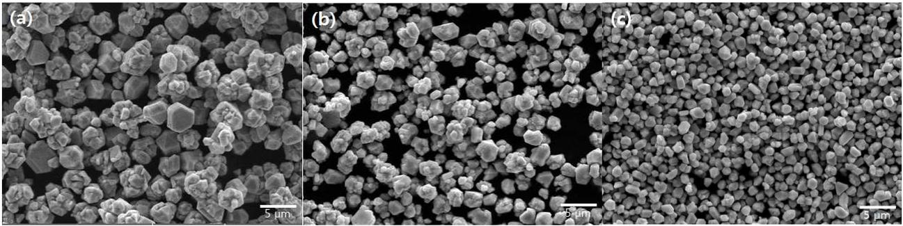
Fig. 3. SEM images of Cu particles synthesized with different amounts of gelatin at 90 °C: (a) 2, (b) 4, and (c) 6 g.
