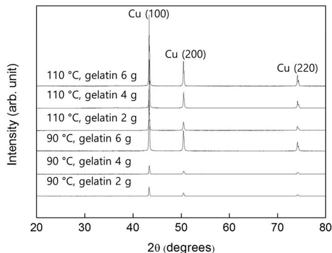
Fig. 2. XRD results of particles synthesized with different temperatures and amounts of gelatin.
