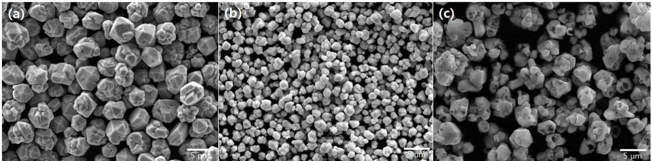
Fig. 4. SEM images of Cu particles synthesized with different amounts of gelatin at 110 °C: (a) 2, (b) 4, and (c) 6 g.
