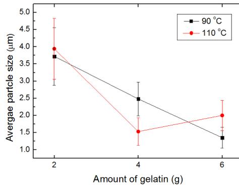
Fig. 5. Particle size distribution of Cu particles synthesized with different temperatures and amounts of gelatin.
