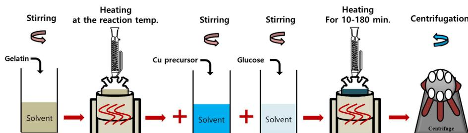
Fig. 1. Fabrication procedure for green synthesizing Cu powders with particle sizes of several micrometers.
