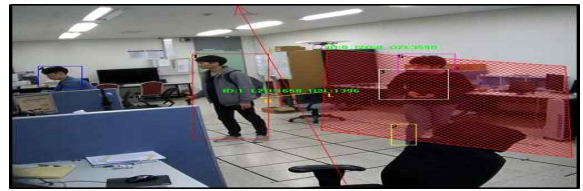
Fig. 2. Example of trip wire and intruder detection
