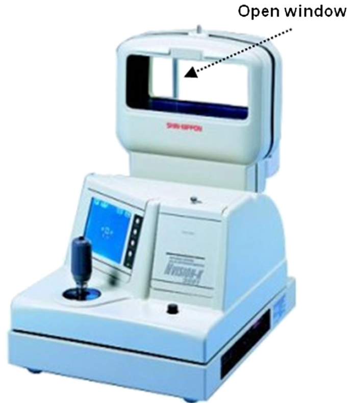
FIGURE 3 — Autorefractometer with the open binocular field of view: Shin-Nippon Nvision—K 5001. Through the open window, the participant can observe the stereoscopic display.
