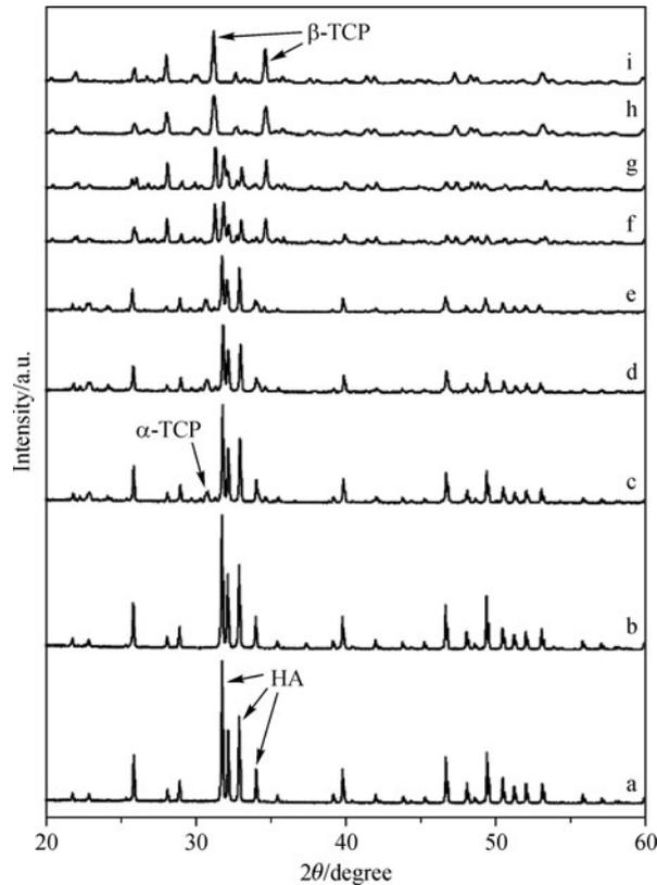
**Fig. 3** XRD patterns of 1250°C sintered Si–HA samples: pure HA (a); 0.4 wt.% Si–HA (b); 0.8 wt.% Si–HA (c); 1.2 wt.% Si–HA (d); 1.6 wt.% Si–HA (e); 2 wt.% Si–HA (f); 3 wt.% Si–HA (g); 4 wt.% Si–HA (h); 5 wt.% Si–HA (i). (Reproduced with permission from Ref. [11], Copyright 2012 IOP Publishing Ltd.)
