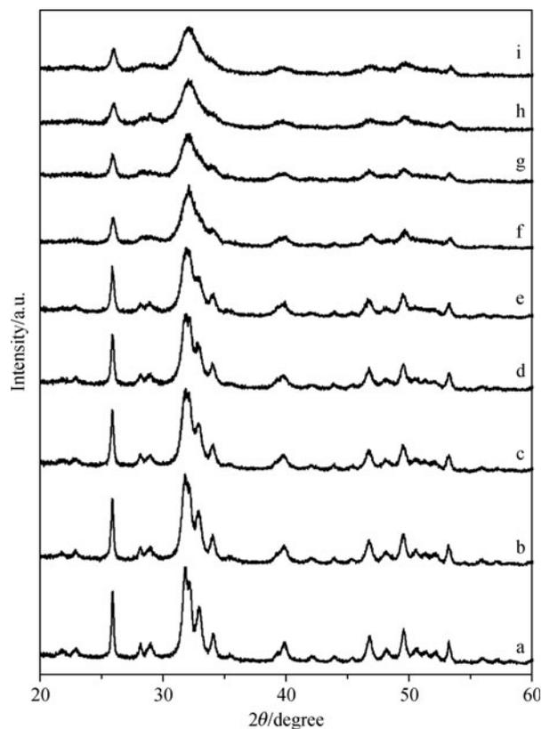
**Fig. 2** XRD patterns of as-prepared Si-HA samples: pure HA (a); 0.4 wt.% Si-HA (b); 0.8 wt.% Si-HA (c); 1.2 wt.% Si-HA (d); 1.6 wt.% Si-HA (e); 2 wt.% Si-HA (f); 3 wt.% Si-HA (g); 4 wt.% Si-HA (h); 5 wt.% Si-HA (i). (Reproduced with permission from Ref. [11], Copyright 2012 IOP Publishing Ltd.)
