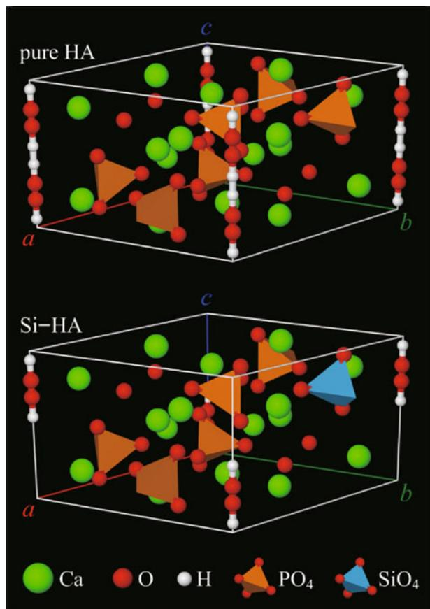
**Fig. 1** Schematic presentation of the cell lattice comparison between pure HA and Si-HA. The loss of the hydroxyl group indicates the decrease of occupancy, since the substitution of  $\text{SiO}_4^{4-}$  for  $\text{PO}_4^{3-}$ . (Reproduced with permission from Ref. [11], Copyright 2012 IOP Publishing Ltd.)
