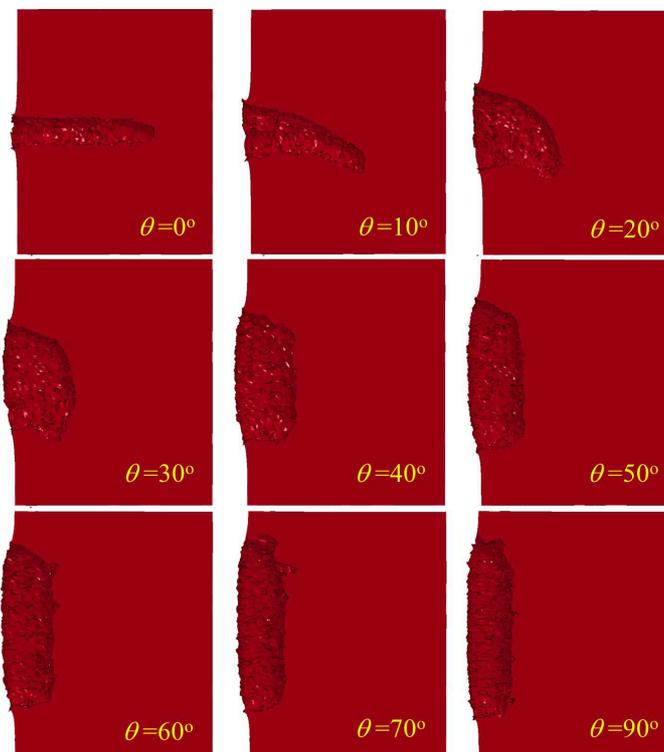
Figure 3 Shapes of the penetration holes for varying obliquity of the penetrator.
