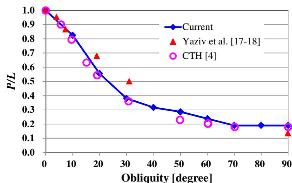
Figure 4 Depth of penetration in the RHA witness block by the WHA long-rod penetrator ( $L/D=10$ ;  $V=1.4$  km/sec) with varying obliquity.
