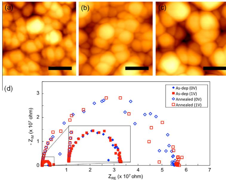
**Figure 3.** AFM images of 200 nm-thick YDC films: (a) as-deposited, (b) annealed at 1000 °C, and (c) annealed at 1200 °C. Scale bars are 100 nm. (d) Sample EIS spectra of as-deposited and 1000 °C-annealed YDC films at 0 V and 1 V. Inset is the zoomed-in plot for  $0 < Z_{RE} < 4E6$  (ohm), and  $0 < -Z_{IM} < 2E6$  (ohm).
