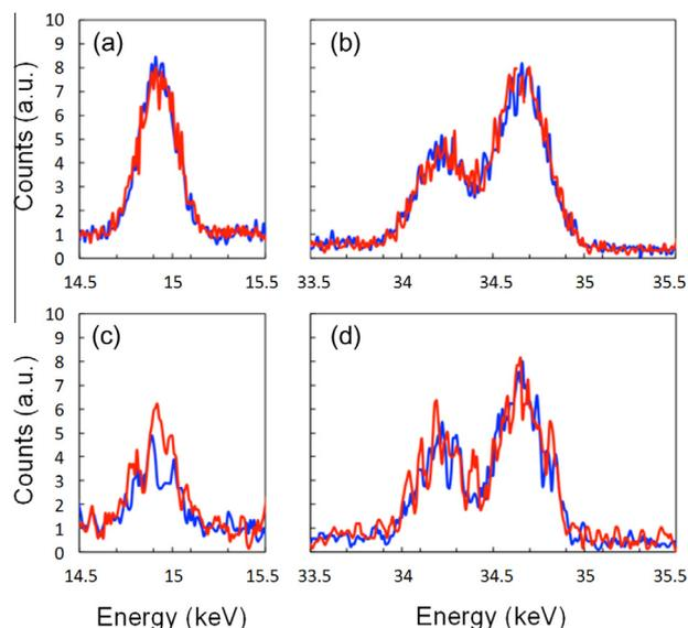
**Figure 2.** EDS spectra of YDC samples near (a) the Y-Kα edge and (b) the Ce-Kα edge in the as-deposited sample, and (c) the Y-Kα edge and (d) the Ce-Kα edge in the annealed sample. Spectra in red are from grain boundaries, and those in blue are from grain centers. (For interpretation of the references to color in this figure legend, the reader is referred to the web version of this article.)
