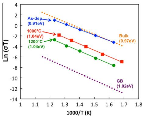
**Figure 4.** Arrhenius plot of as-deposited, 1000 °C-annealed, and 1200 °C-annealed samples (12 mol% YDC). Reference data for dotted-lines, which represent the bulk (i.e., epitaxial), and grain-boundary conductivities for 10 mol% YDC are from Ref. [19].
