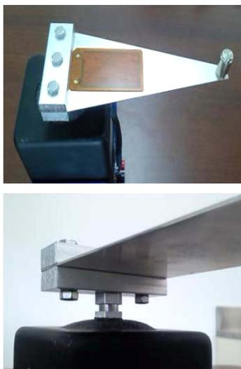
**Fig. 5.** Piezoelectric cantilever set up on top of electromagnetic shaker.
