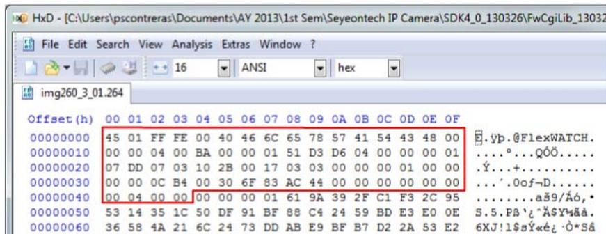
Figure 7. Contents of a sample IP camera packet, P-frame with manufacturer header
