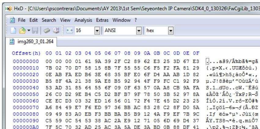
Figure 8. Contents of a sample IP camera packet, P-frame, manufacturer header removed
