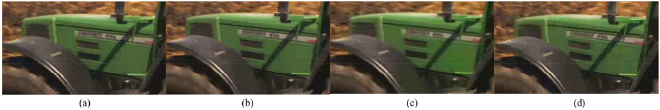
Fig. 9. Still images of the reconstructed “Tractor” video sequences for the low bitrate. (a) Conventional VRS. (b) LWC VRS. (c) LWC + DS VRS. (d) Low-power H.264 VRS.
