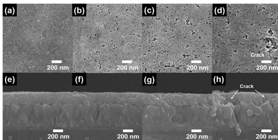
Fig. 2 (a–d) Top-view and (e–h) cross-view FESEM images of bare  $WO_3$ ,  $WO_3$ -0.5RP,  $WO_3$ -1RP, and  $WO_3$ -5RP, respectively.
