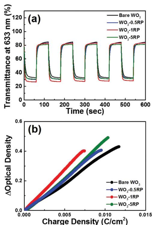
Fig. 5 (a) *In situ* optical transmittance curves of all samples traced in the stepping potential at -0.7 V for the coloured state and 1.0 V for the bleached state for 60 s and (b) optical density variation at 633 nm with respect to the inserted charge density.
