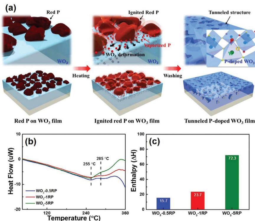
**Fig. 1** (a) Schematic diagram of the formation process for the tunneled P-doped  $\text{WO}_3$  films using ignited red P, (b) DSC curves obtained from the  $\text{WO}_3$  films with different weight percentages of red P in the temperature range of 25 to 360 °C, and (c) histograms of enthalpy values calculated using the exothermic peak of 255–285 °C.
