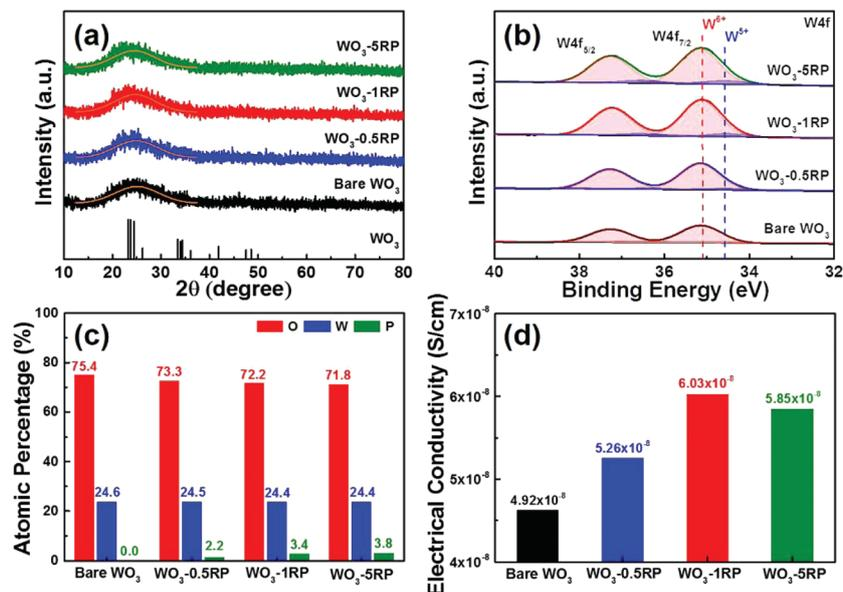
Fig. 3 (a) XRD patterns, (b) W 4f XPS core-level spectra, and histograms of (c) atomic percentages for W, O, and P elements and (d) electrical conductivity of all samples.
