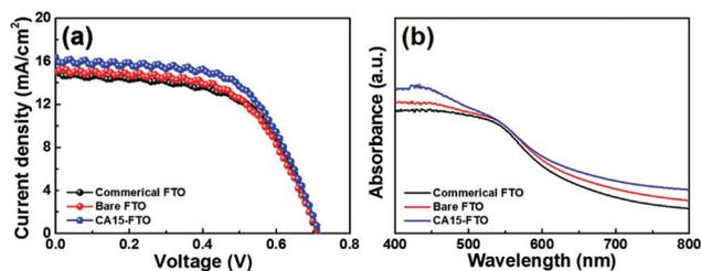
Fig. 7 (a) Photocurrent–voltage ( $J$ – $V$ ) curves measured from the DSSCs using the commercial FTO, bare FTO, and CA15-FTO as a TCO of the working electrode and (b) absorption spectra of the half cells with the FTO films and  $\text{TiO}_2$  with the dye.
