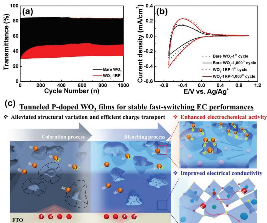
**Fig. 6** (a) Variation of *in situ* optical transmittance modulation at 633 nm for bare  $\text{WO}_3$  and  $\text{WO}_3$ -1RP during continuous CV cycling (1000 cycles) showing the EC cycling stability, (b) comparison of CV curves obtained from the 1<sup>st</sup> (dashed line) and 1000<sup>th</sup> cycle (solid line) for bare  $\text{WO}_3$  and  $\text{WO}_3$ -1RP, and (c) a possible mechanism of the improved EC performance using the tunneled P-doped  $\text{WO}_3$  films.
