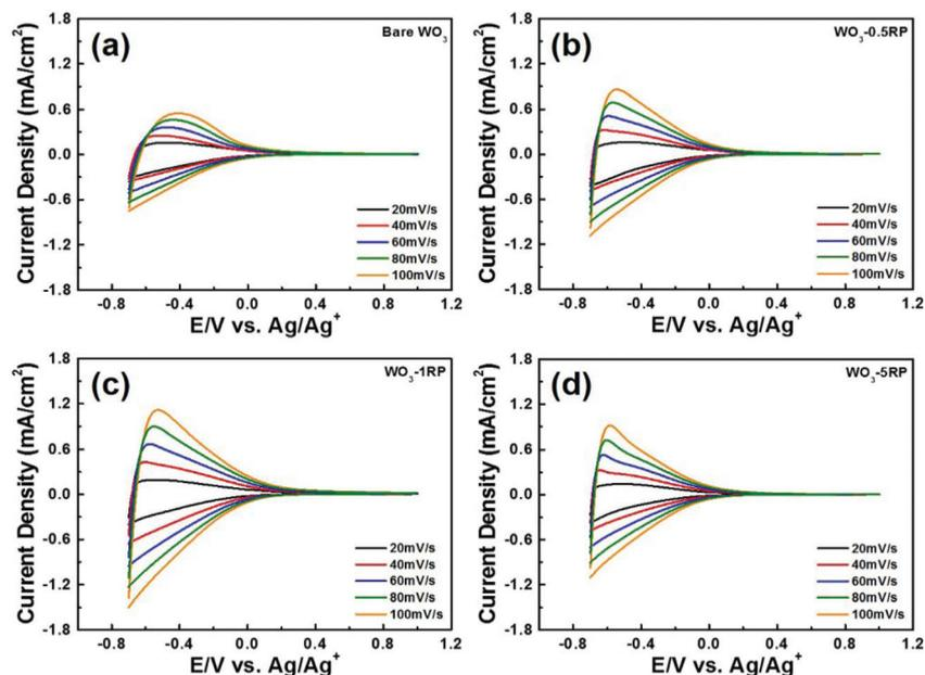
Fig. 4 (a–d) CV curves of all samples recorded between  $-0.7$  and  $1.0$  V at the varied scan rate from  $20$  to  $100$  mV s<sup>-1</sup> using the three-electrode system.
