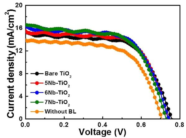
**Fig. 6.** (a)  $J$ - $V$  curves of the DSSCs with the Nb- $\text{TiO}_2$  BLs prepared by the varied Nb/Ti molar ratios and without BL.
