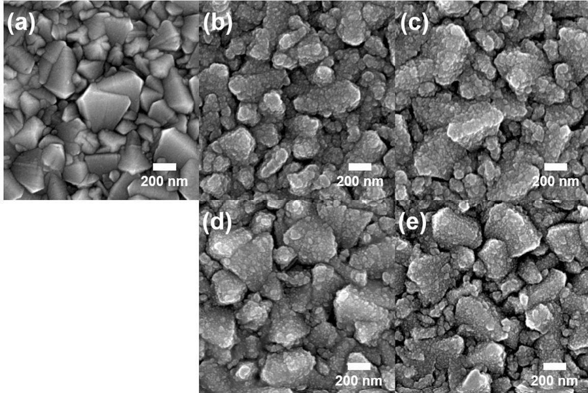
**Fig. 1.** Top-view FESEM images of (a) only FTO glass, (b) bare  $\text{TiO}_2$ , (c) 5Nb- $\text{TiO}_2$ , (d) 6Nb- $\text{TiO}_2$ , and (e) 7Nb- $\text{TiO}_2$ .
