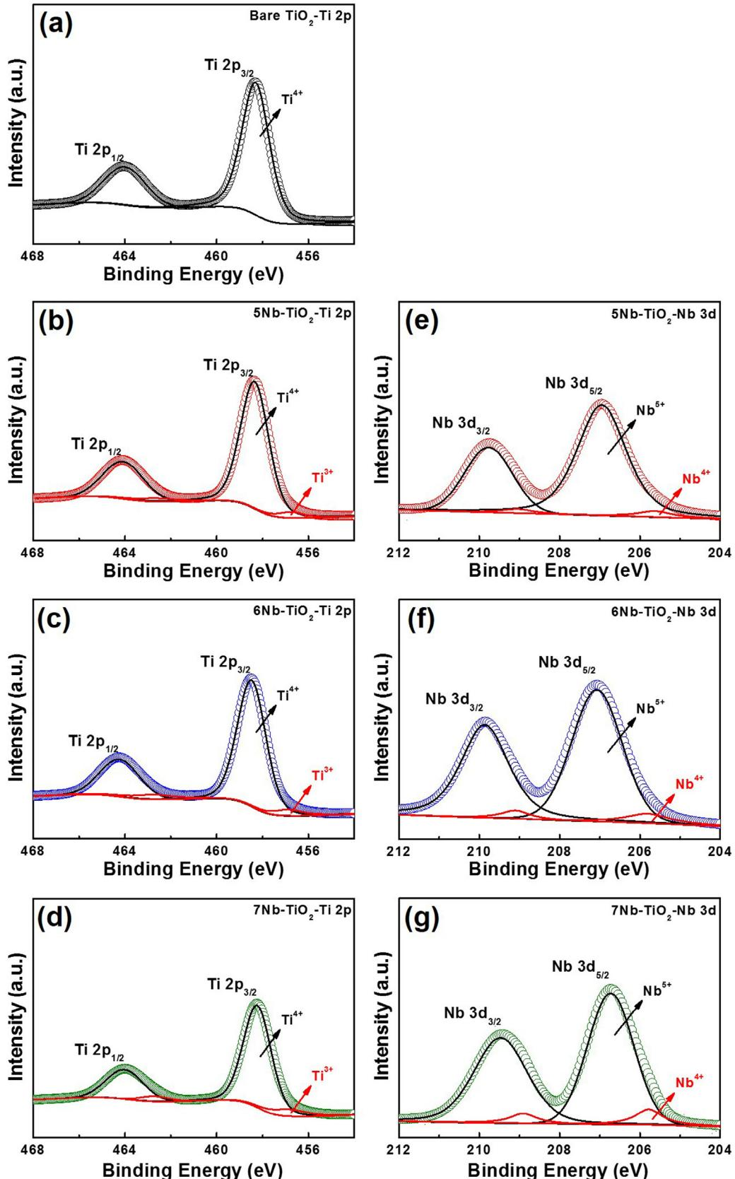
Fig. 3. XPS core-level spectra of (a) Ti 2p obtained from bare TiO<sub>2</sub> and (b-d) Ti 2p and (e-g) Nb 3d obtained from 5Nb-TiO<sub>2</sub>, 6Nb-TiO<sub>2</sub>, and 7Nb-TiO<sub>2</sub>.
