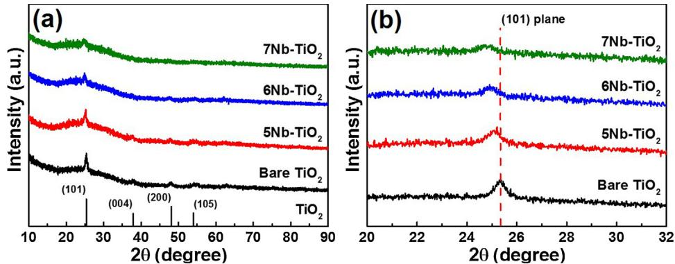
**Fig. 2.** (a) XRD pattern of bare  $\text{TiO}_2$ , 5Nb- $\text{TiO}_2$ , 6Nb- $\text{TiO}_2$ , and 7Nb- $\text{TiO}_2$ . (b) the detailed XRD pattern of the (101) peak.
