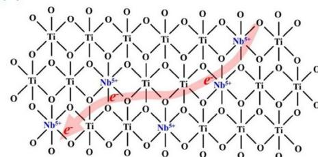
**Fig. 7.** Schematic of two main effects for high-performance DSSCs in the Nb-TiO<sub>2</sub> BLs.
