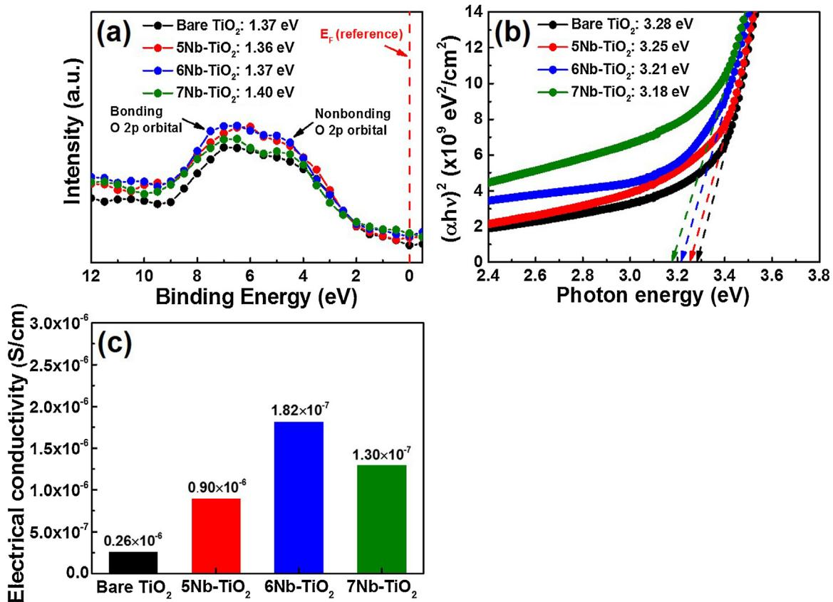
**Fig. 4.** (a) Valence band XPS spectra, (b) plots of  $(ahv)^2$  versus photon energy, and (c) electrical conductivity of the Nb-TiO<sub>2</sub> BLs with Nb/Ti molar ratio of 0, 5, 6, and 7.
