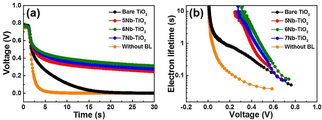
**Fig. 5.** (a) OCVD curve of the DSSCs with bare  $\text{TiO}_2$ , 5Nb- $\text{TiO}_2$ , 6Nb- $\text{TiO}_2$ , and 7Nb- $\text{TiO}_2$  and without the BLs. (b) Comparison of electron lifetime among the samples as a function of voltage.
