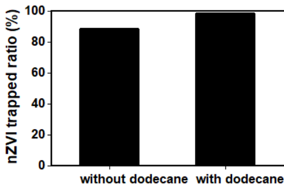
Fig. 12. PVP/VA-nZVI trapped ratio with and without dodecane layer.
