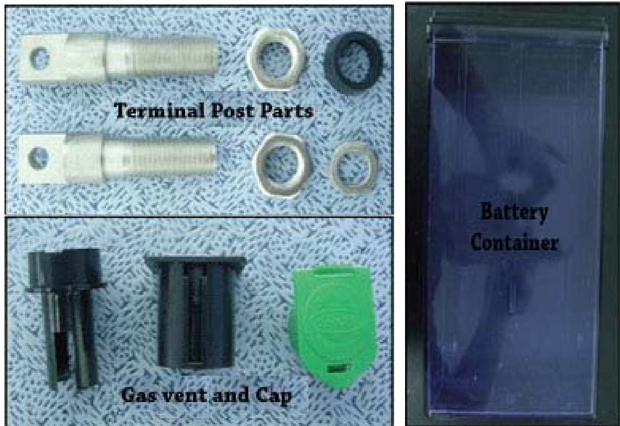
Fig. 3. Components of the Ni-Zn pocket-type battery and battery container.
