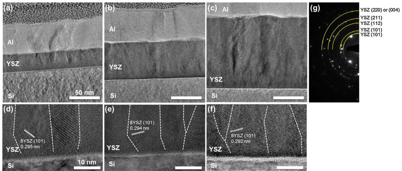
**Fig. 2.** ((a)–(f)) Cross-sectional TEM images of ALD YSZ films at low magnification ((a) 35 nm, (b) 61 nm, and (c) 138 nm samples) and at high magnification near the YSZ-Si interface ((a) 35 nm, (b) 61 nm, and (c) 138 nm samples), and (g) the SAD pattern of the 138 nm sample.
