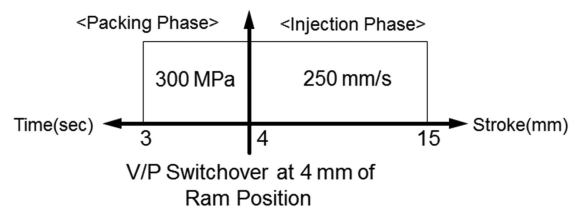
Figure 4. Injection Molding Condition for Pyramidal Kagome Core Strip.
