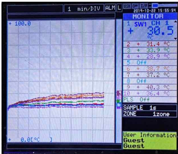
Fig. 13. Thermal test of switches in FDC.
