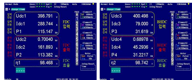
Fig. 11. Measured efficiency at full load.
