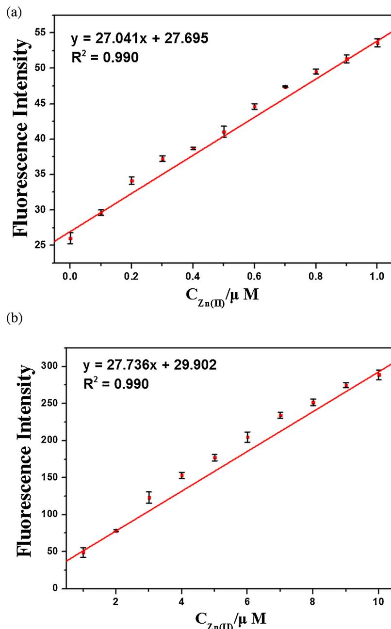
**Fig. 4.** Fluorescence intensity (at 500 nm) of **1** as a function of Zn(II) concentration. (a)  $[1] = 10 \mu\text{mol/L}$ ,  $[\text{Zn(II)}] = 0\text{--}1.00 \mu\text{mol/L}$ ; (b)  $[1] = 20 \mu\text{mol/L}$ ,  $[\text{Zn(II)}] = 1.00\text{--}10.00 \mu\text{mol/L}$ . Conditions: all samples were conducted in buffer–MeOH solution (999:1, 10 mM bis–tris, pH 7.0).  $\lambda_{\text{ex}}$  and  $\lambda_{\text{em}}$  were 356 and 500 nm, respectively.
