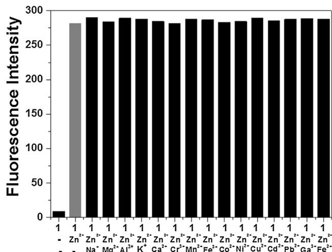
**Fig. 2.** Competitive selectivity of **1** (10  $\mu$ M) toward Zn<sup>2+</sup> (1 equiv) in the presence of other metal ions (1 equiv) with an excitation of 356 nm in buffer solution (10 mM bis-tris, pH 7.0).
