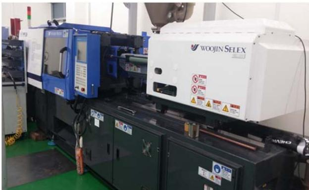
**Figure 6.** Picture of Injection molding machine used in this study.
