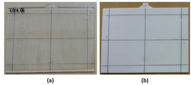
Figure 17. Injection molded for model-1. (a) PC, (b) PBT
