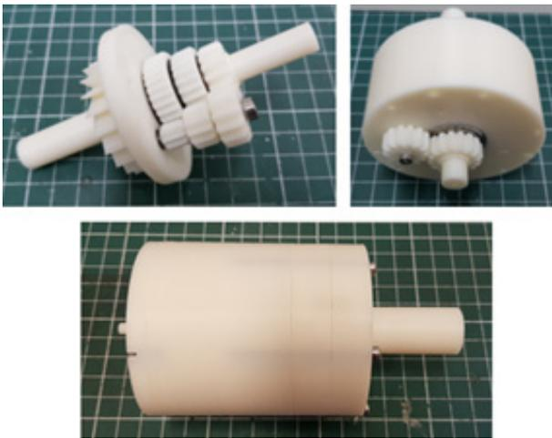
Fig. 15 Multiple bearing module assembly
