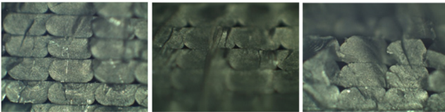
(b) Optical micrograph ( \times 100 ) of the specimen fabricated at 245 °C, 260 °C, and 275 °C from left to right
