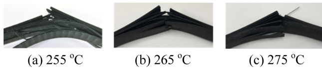
Figure 8. Fractured PC-24 specimen fabricated by ME-type 3D printing at various nozzle temperatures after cooling using liquid nitrogen.
