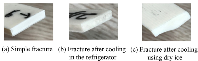
Figure 4. Fractured ABS specimen fabricated by ME-type 3D printing at a nozzle temperature of 250 °C.
