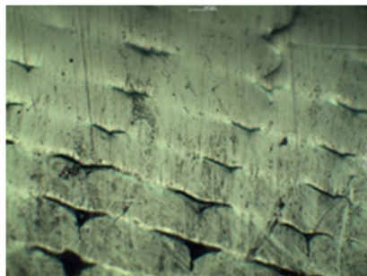
(a) Fracture after cooling in the refrigerator
