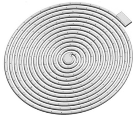
Figure 2. Shape of spiral specimen (ASTM D 3123).
