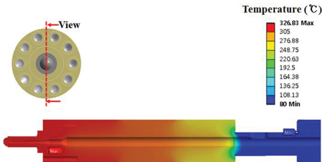
Figure 7. Temperature distribution of the bimetal cylinder.
